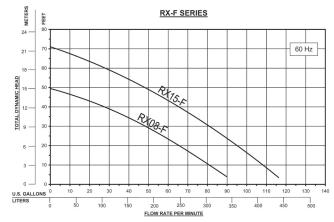
**PORTABLE TOP DISCHARGE:** 2", to 110 gpm, 70 ft head **RX-F** Series: All 316SS
