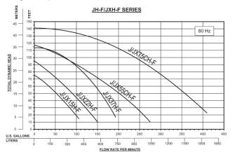
SUMP PUMPS: 2-4", to 650 gpm and 140 ft head
