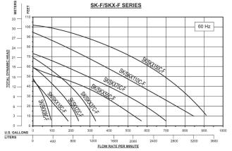
SHREDDER PUMPS: 2 - 6", to 900 gpm, 100 ft head
