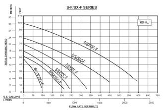
NON-CLOG PUMPS: 2 - 4", to 600 gpm, 140 ft head S-F Series: Cast Iron / 304SS • \$X-F Series: All 316SS
