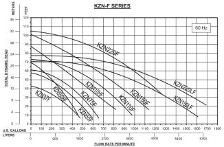
**SLURRY PUMPS:** 3-6", to 1690 gpm, 105 ft head **KZN-F** Series: Hi Chrome / Cast Iron
