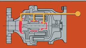
Patented PPS bushing and superior design help guard against premature heat damage should the pump run dry or be operated against a closed valve.
